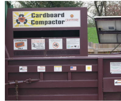
Solar-powered cardboard compactor at the Municipal Center.
